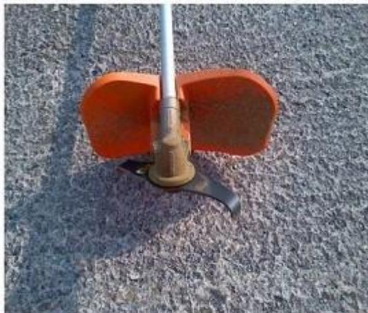
Figure 1 - Stihl brush cutter with shredder blade and correct protective guard fitted.
